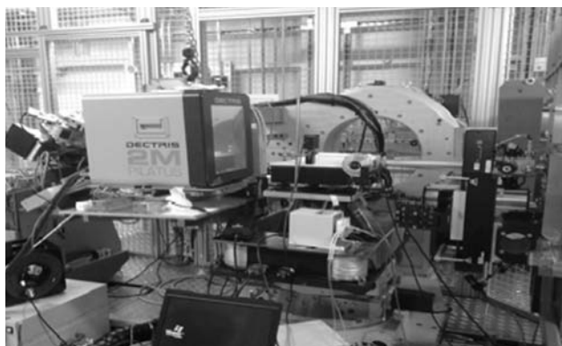
The I07 diffractometer in an alternative mode of operation. The detachable sample stage has been removed and the hexapod has been mounted in such a way that it supports a horizontally oriented sample cell for liquid interface experiments. The Pilatus 2M has also been mounted, via a detachable platform, to the diffractometer's detector arm.
