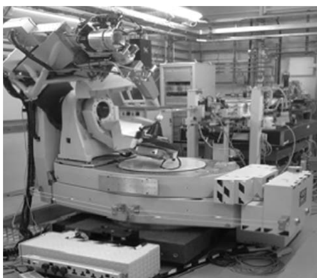
The layout of the experiments hutch of beamline I16. The 6-circle geometry diffractometer is shown in the foreground while the optics table is shown in the background.
